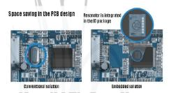
For the past several decades, quartz crystal based oscillators, clock generators and resonators were the primary reference timing components in electronics, since there were no real alternatives. Recently a new technology rose up, offering the first devices where the MEMS structures are built in the same package with the analog circuitry.
